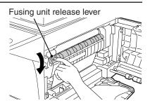
Gently remove the misfed paper from under the fusing unit as shown in the illustration. If the paper cannot
